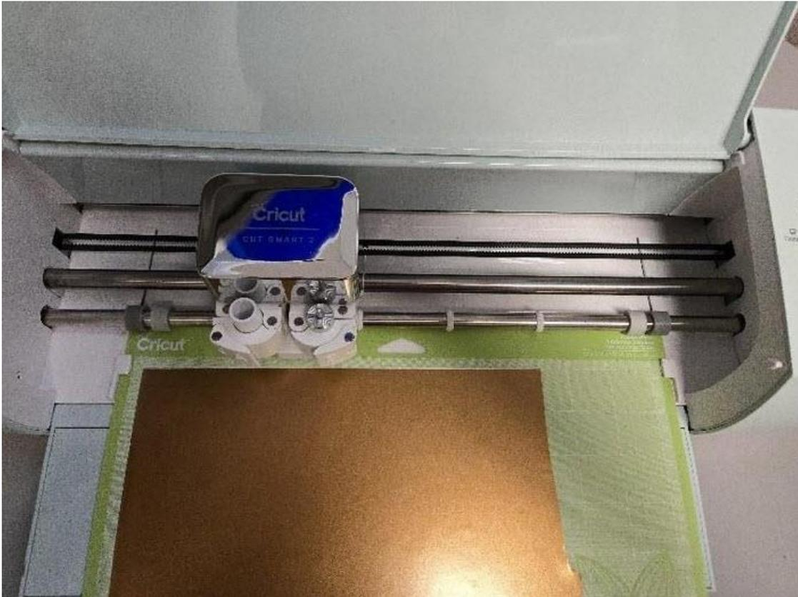
4. Press the carrier sheet load button.
