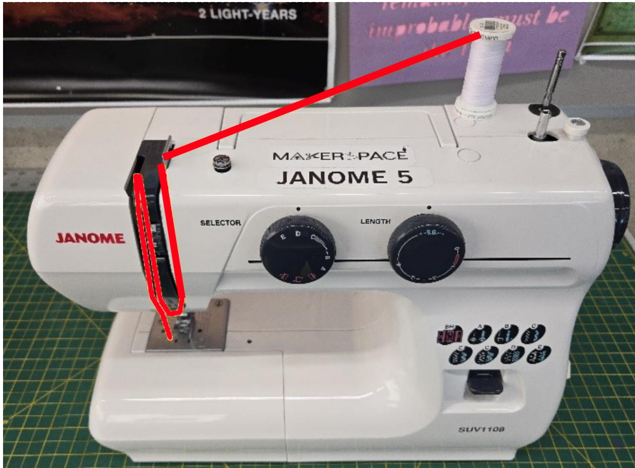
A photograph showing how to load the thread.
