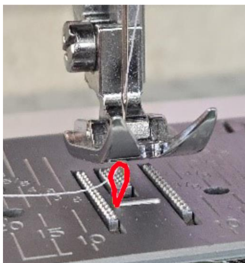
A photograph showing how the bobbin thread will appear as a loop.
