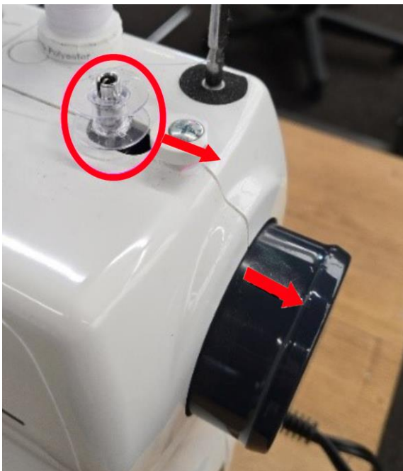
A photograph showing how to pull the handwheel outward and push the bobbin on the holder to the right.
