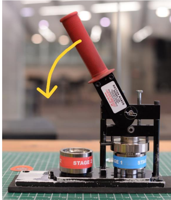
A photograph showing how to rotate stage one and push down to join the layers.
