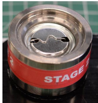
Two photographs showing how to place the backing in stage 2, zigzag side facing up for pinback buttons, and open side facing down for magnets.
