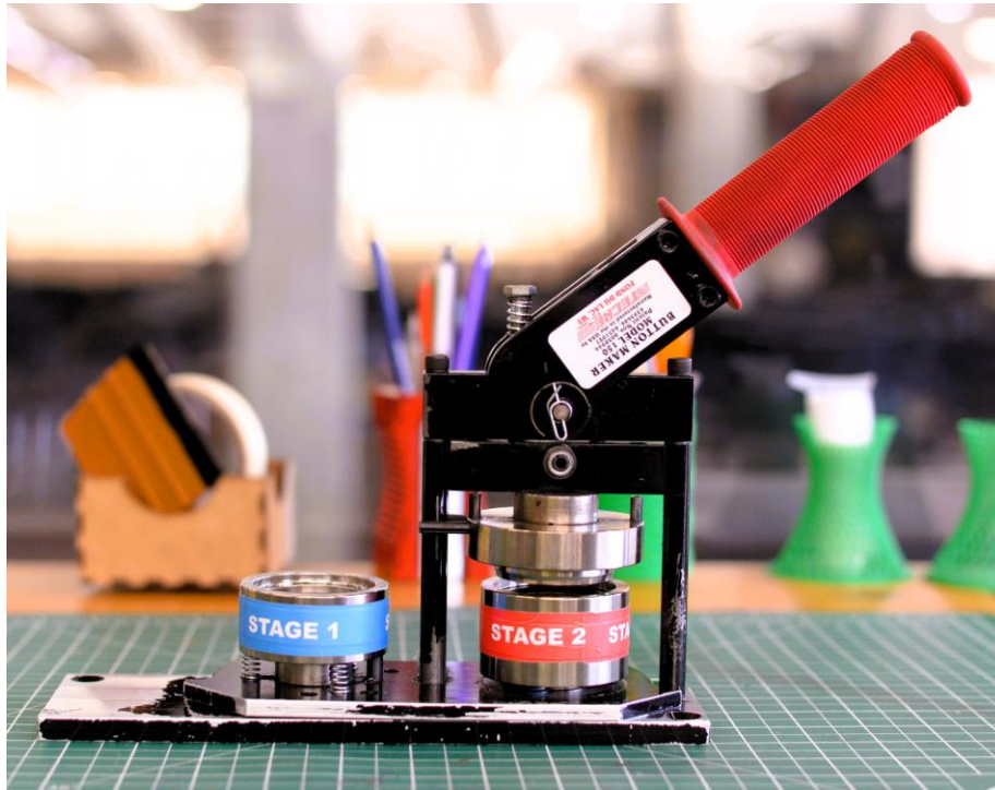
A photograph of the button maker, showing stage 1 and stage 2 on the rotating base.
