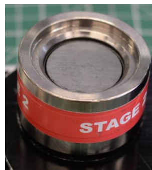
Two photographs showing how to place the backing in stage 2, zigzag side facing up for pinback buttons, and open side facing down for magnets.
